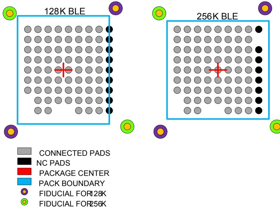
The rightmost column of (all NC, No Connect) balls in the 256K BLE WLCSP is for mechanical integrity purposes. The package is thus wider (3.2 mm versus 2.8 mm). All other dimensions are identical. Cypress will provide layout symbols for PCB layout.
