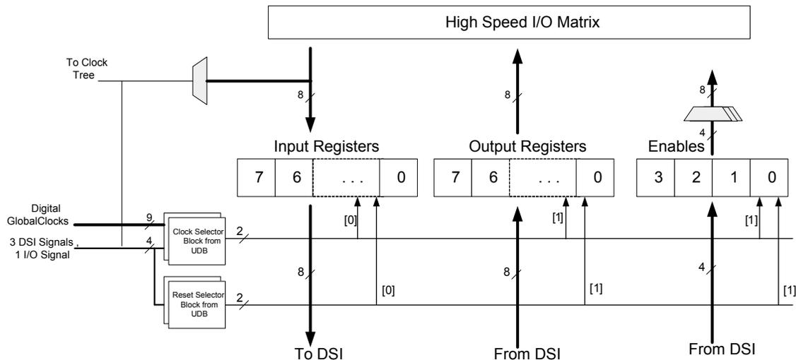
UDBs can generate interrupts (one UDB at a time) to the interrupt controller. UDBs retain the ability to connect to any pin on the chip through the DSI.
