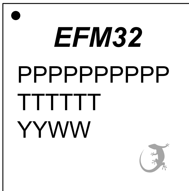
Figure 7.3. BGA125 Package Marking
