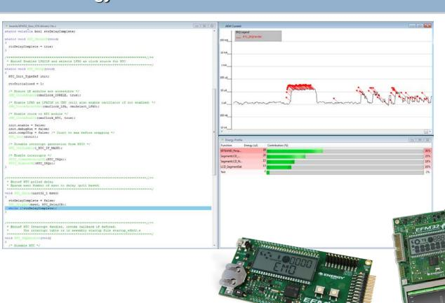
The energyAware Profiler is an energy debugging tool that use Advanced Energy Monitoring (AEM) data available from the development tools to perform real-time profiling and debugging of the associated object code.
