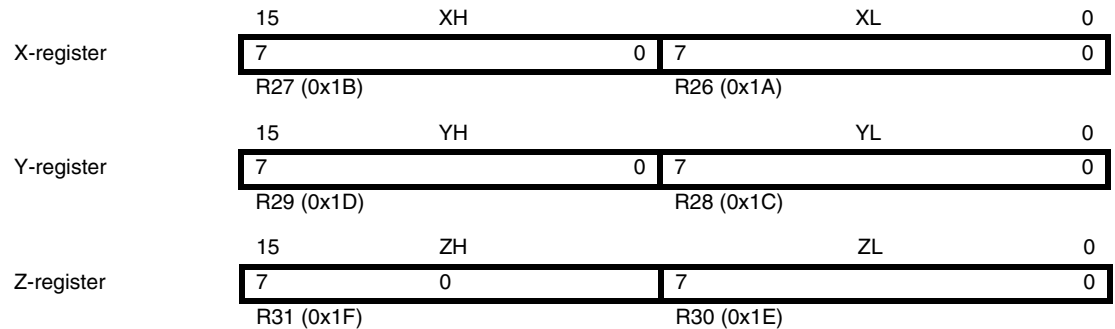
Figure 4-4. The X-, Y-, and Z-registers
