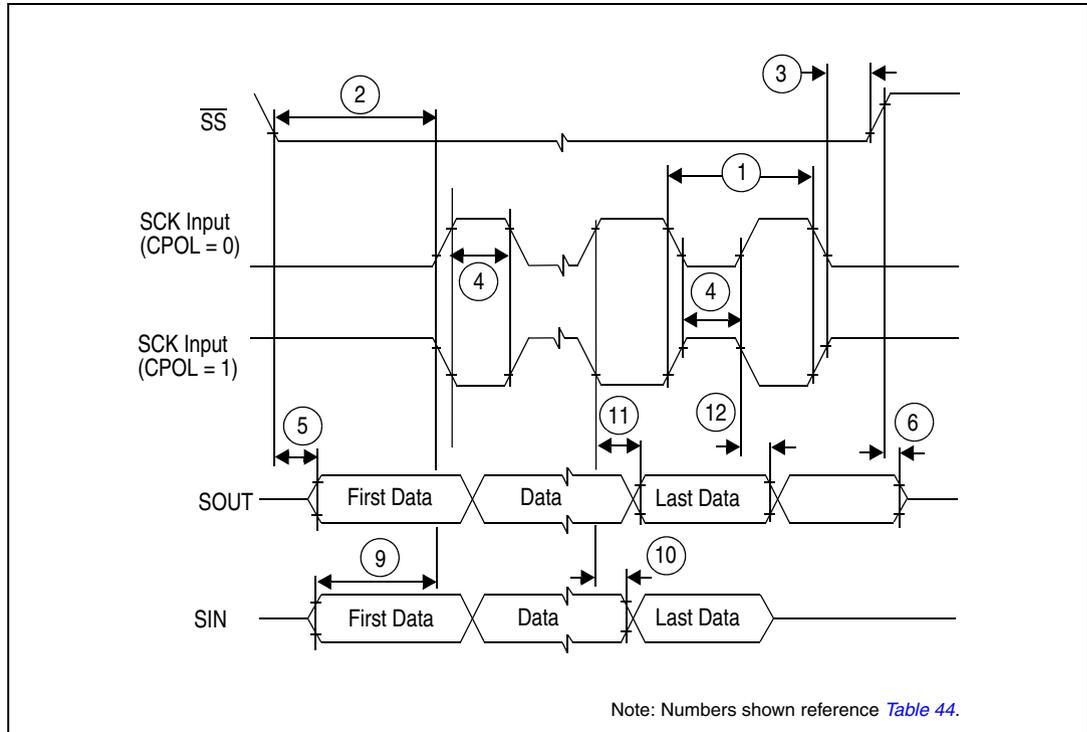
Figure 22. DSPI modified transfer format timing – slave, CPHA = 0
