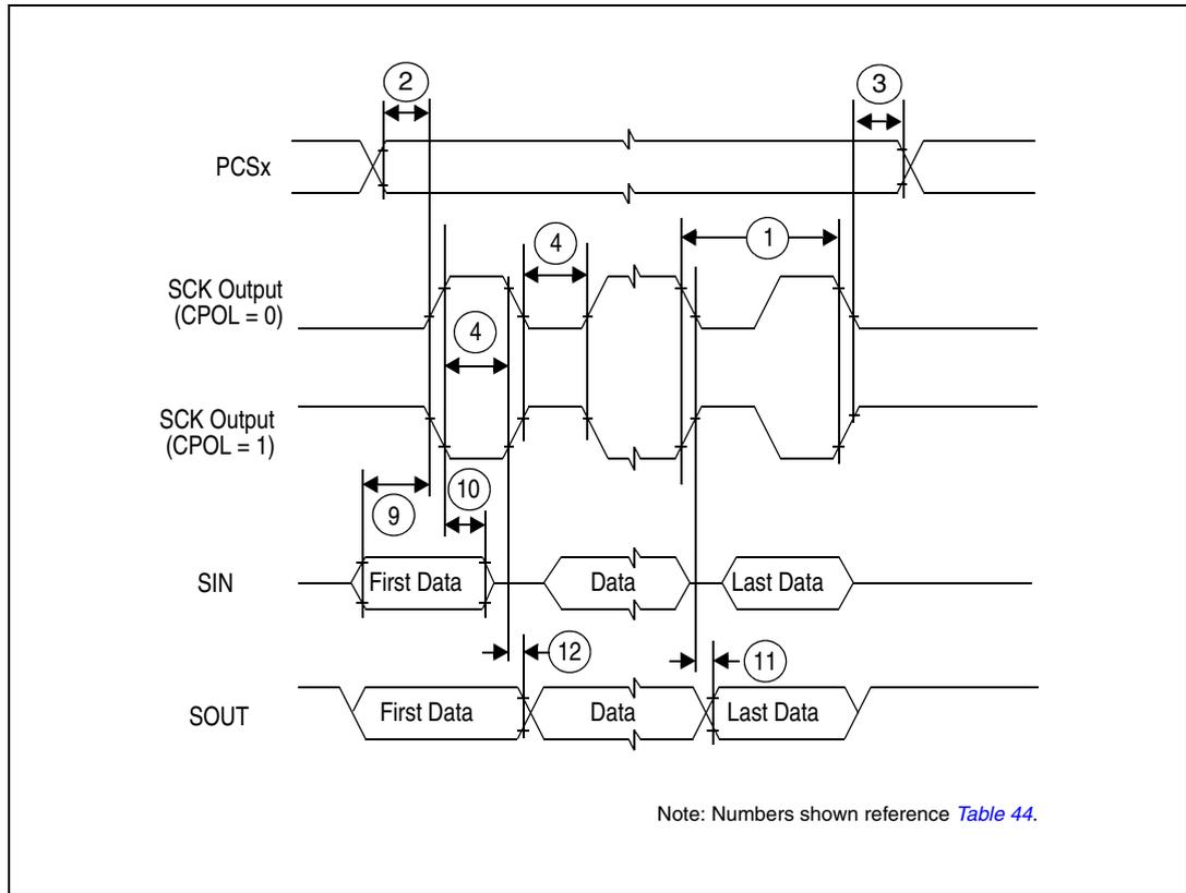
Figure 16. DSPI classic SPI timing – master, CPHA = 0
