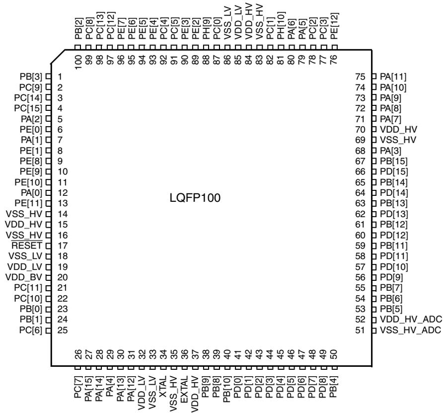
Figure 2. LQFP100 pin configuration (top view)
