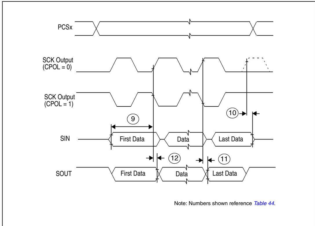
Figure 21. DSPI modified transfer format timing – master, CPHA = 1
