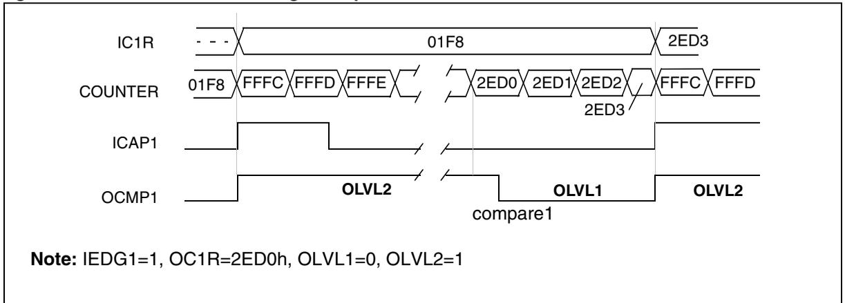
Figure 54. Pulse Width Modulation Mode Timing Example
