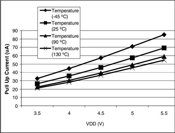
Figure 140. Typical R<sub>PU</sub> vs. V<sub>DD</sub> with V<sub>IN</sub>=V<sub>SS</sub>
