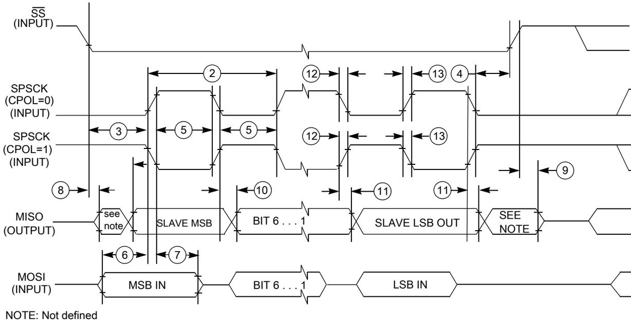
**Figure 16. SPI slave mode timing (CPHA = 0)**
