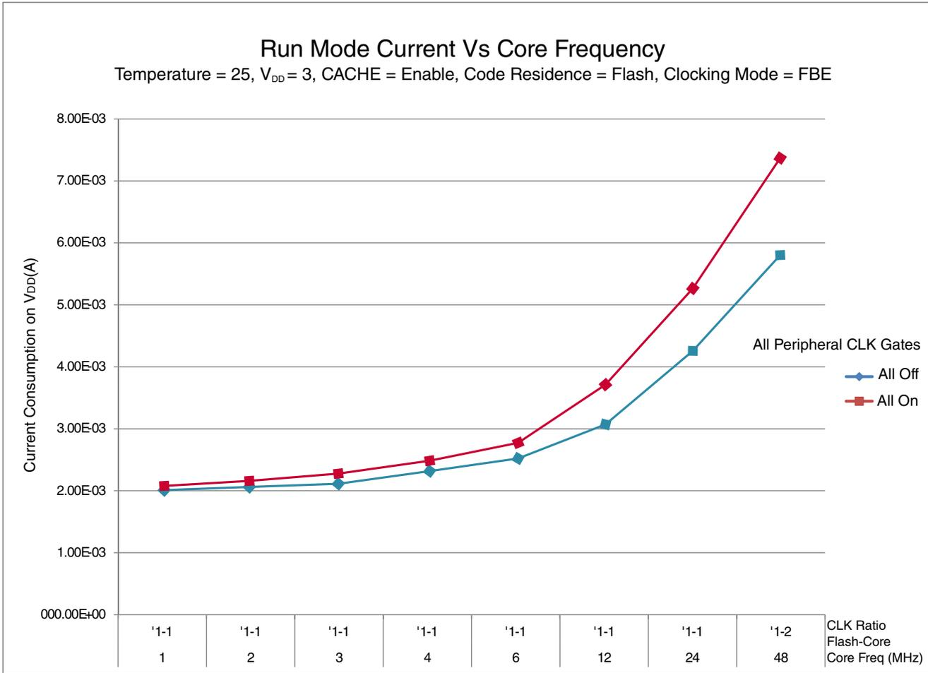
**Figure 3. Run mode supply current vs. core frequency**
