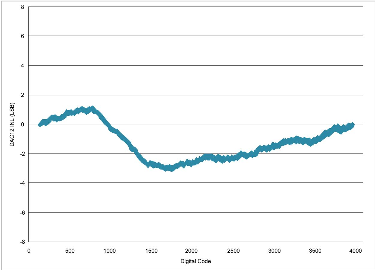
**Figure 12. Typical INL error vs. digital code**
