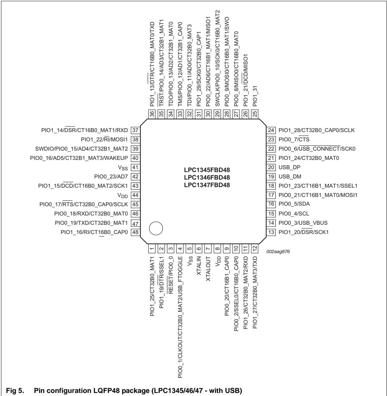
Fig 5. Pin configuration LQFP48 package (LPC1345/46/47 - with USB)
