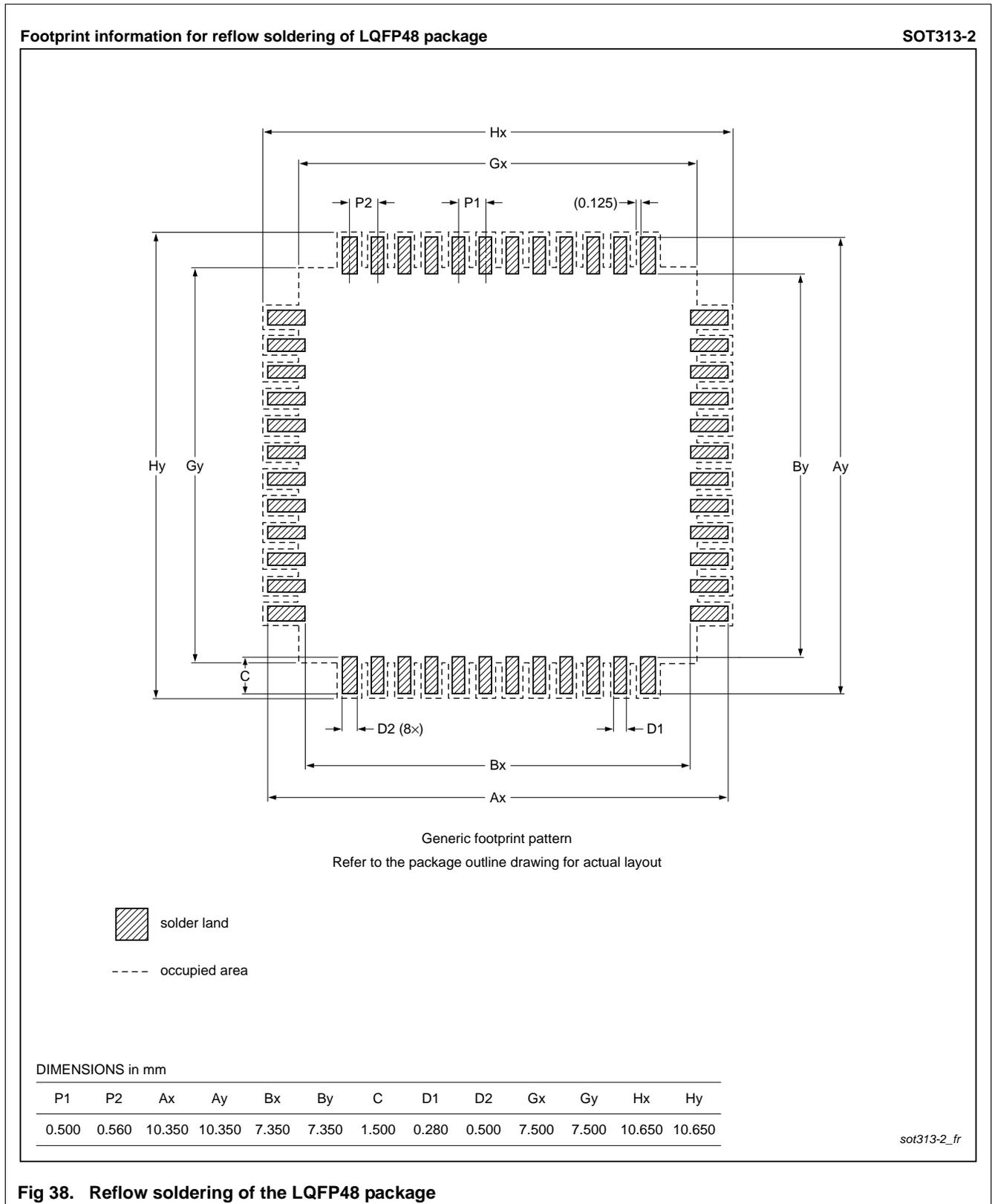
**Fig 38. Reflow soldering of the LQFP48 package**
