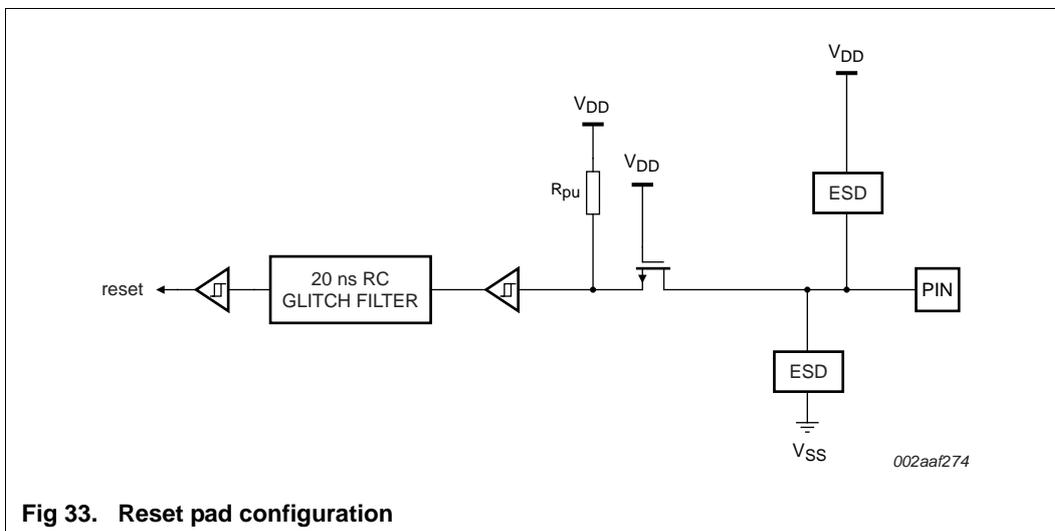
Fig 33. Reset pad configuration
