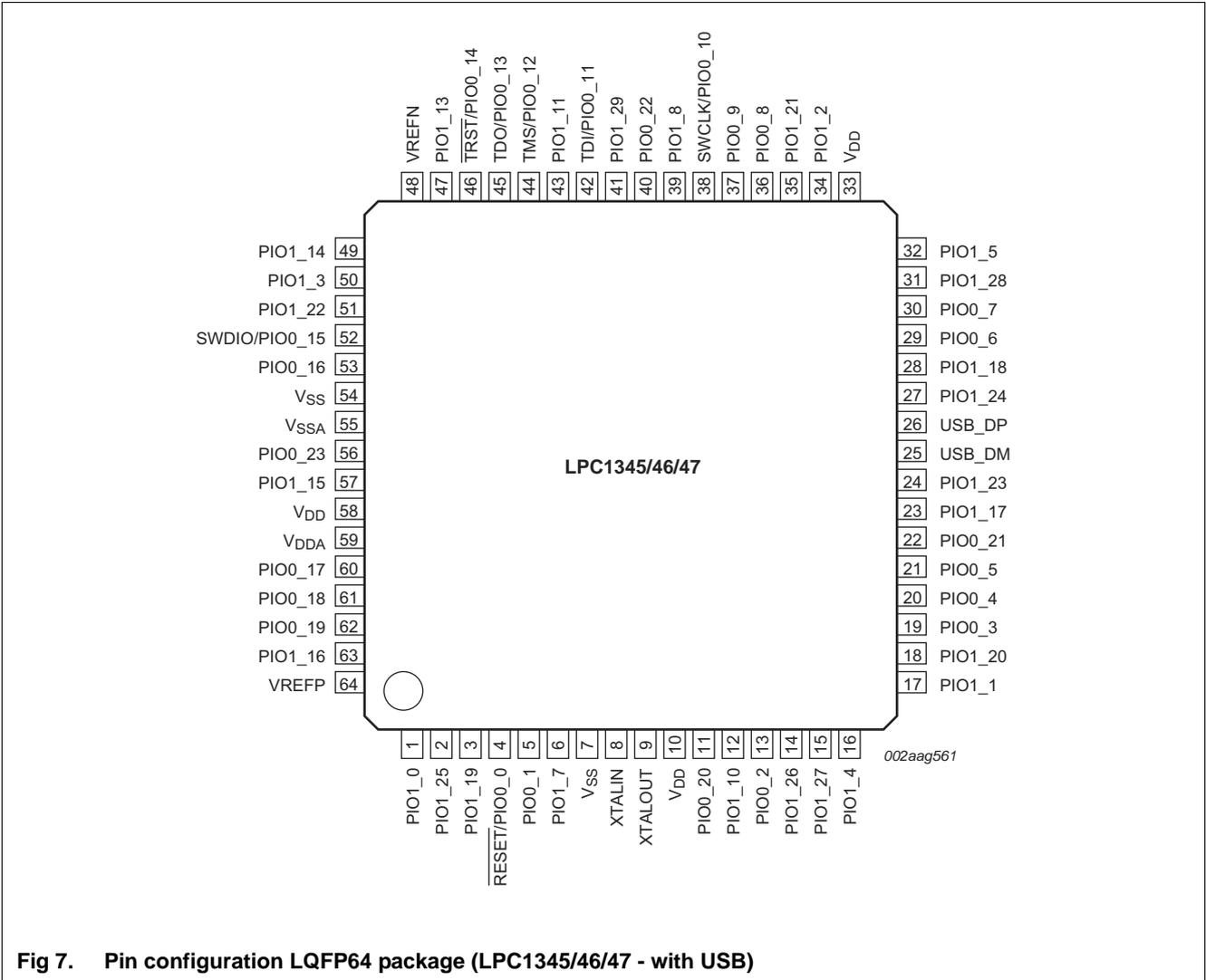
Fig 7. Pin configuration LQFP64 package (LPC1345/46/47 - with USB)
