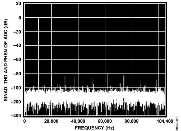
Figure 14. SINAD, THD, and PHSN of ADC, Internal 2.5 V Reference Used
