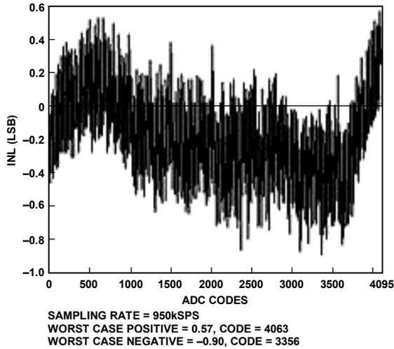
Figure 11. Typical INL,  $f_{ADC} = 950$  kSPS, Internal Reference Used
