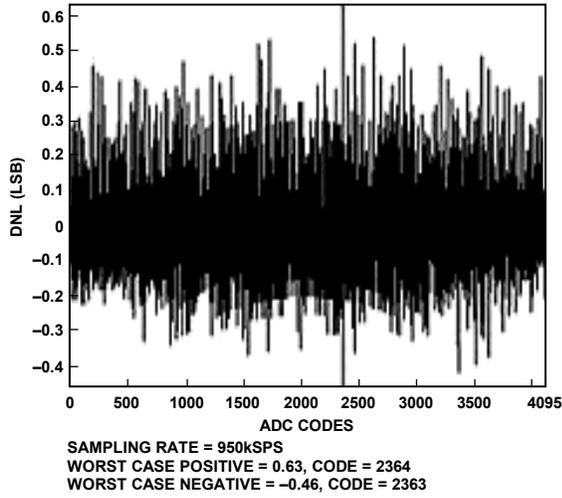
Figure 10. Typical DNL,  $f_{ADC} = 950$  kSPS, Internal Reference Used
