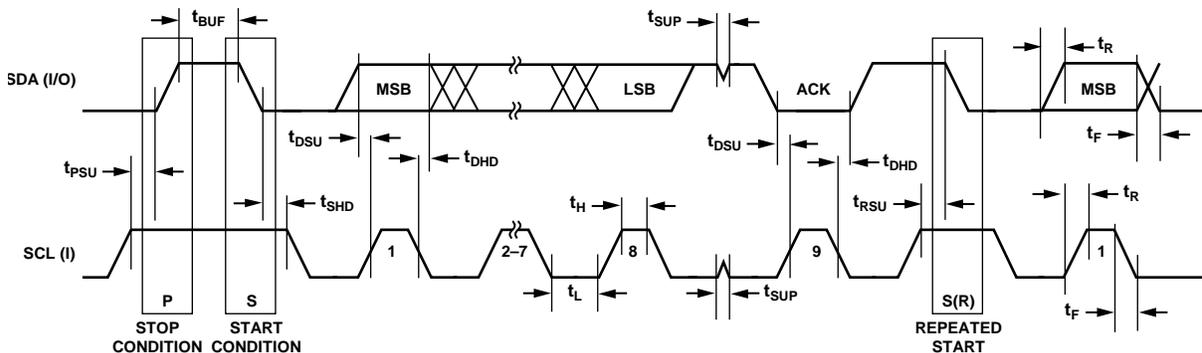
Figure 2. I<sup>2</sup>C-Compatible Interface Timing
