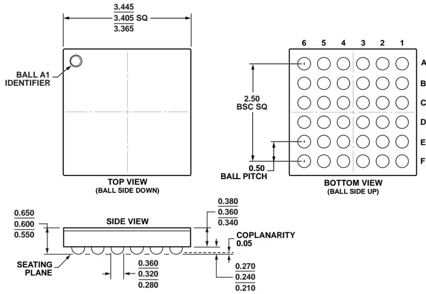
Figure 57. 36-Ball Wafer Level Chip Scale Package [WLCSP]
