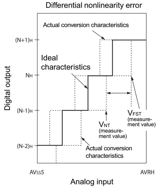
$$\text{Nonlinearity error of digital output } N = \frac{V_{NT} - \{1\text{LSB} \times (N - 1) + V_{OT}\}}{1\text{LSB}} \text{ [LSB]}$$
