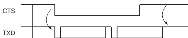
Figure 38-28. Transmitter Behavior when Operating with Hardware Handshaking
