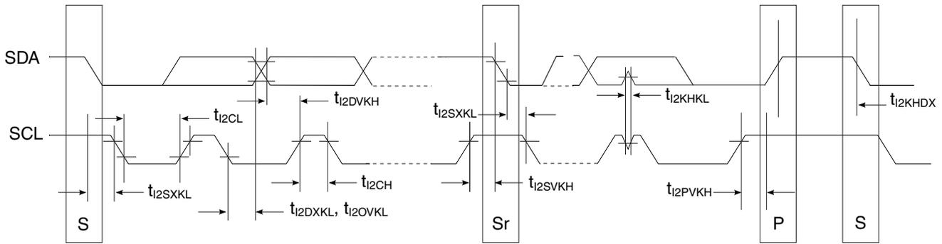
Figure 46. I<sup>2</sup>C bus AC timing diagram
