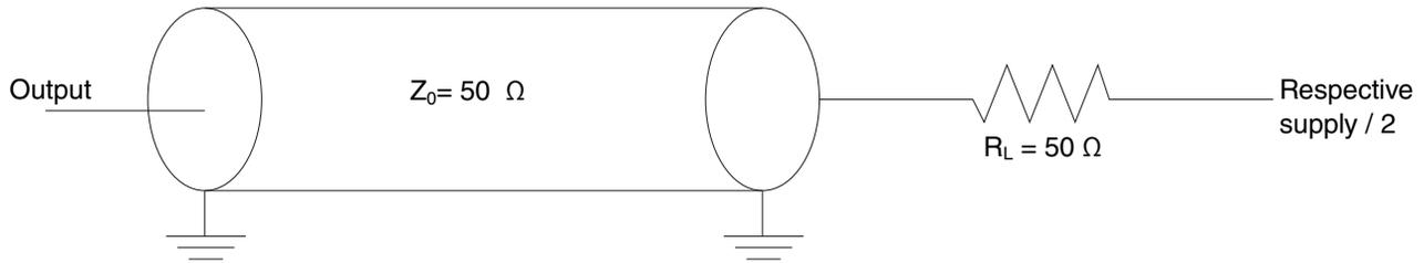
Figure 47. Integrated Flash Controller AC test load
