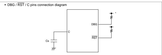
\*: Connect the DBG pin to an external pull-up resistor of 2 k $\Omega$  or above. After power-on, ensure that the DBG pin does not stay at "L" level until the reset output is released. The DBG pin becomes a communication pin in debug mode. Since the actual pull-up resistance depends on the tool used and the interconnection length, refer to the tool document when selecting a pull-up resistor.
