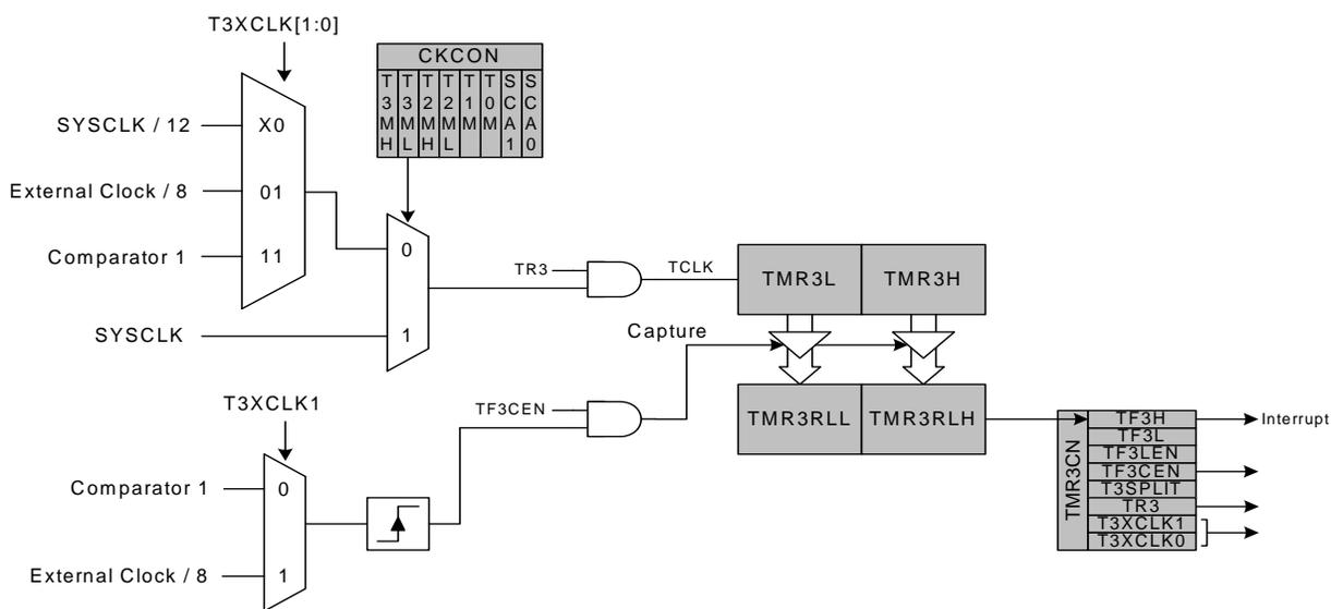
Figure 25.9. Timer 3 Capture Mode Block Diagram
