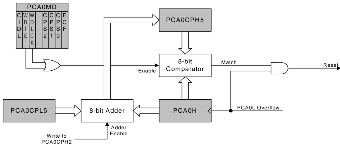
Figure 26.11. PCA Module 5 with Watchdog Timer Enabled
