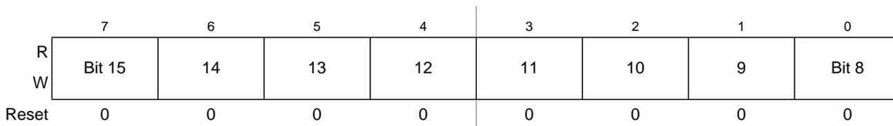
Figure 15-10. TPM Counter Modulo Register High (TPMxMODH)
