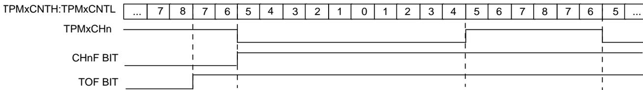
Figure 15-6. Low-True Pulse of a Center-Aligned PWM
