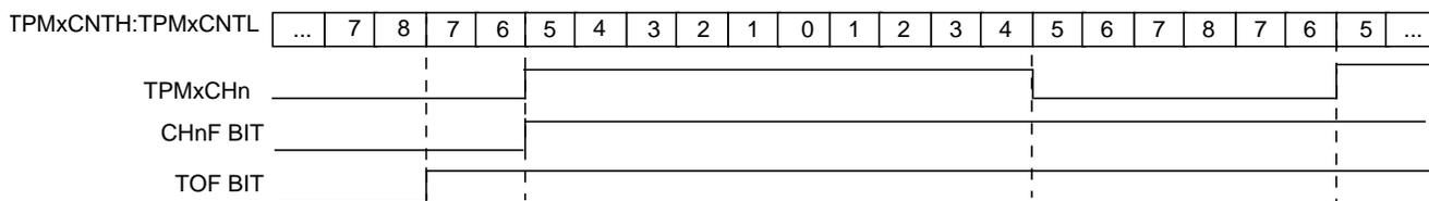
Figure 15-5. High-True Pulse of a Center-Aligned PWM
