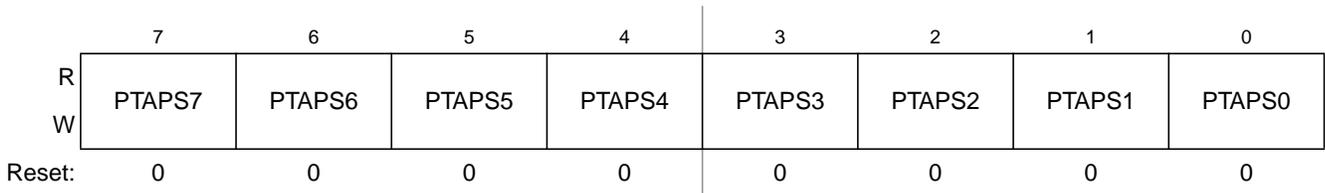
Figure 6-9. Port A Interrupt Pin Select Register (PTAPS)
