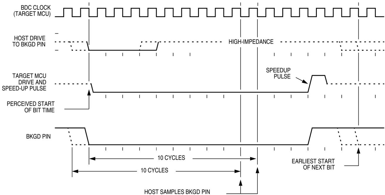
Figure 16-4. BDM Target-to-Host Serial Bit Timing (Logic 0)
