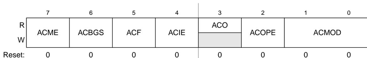
**Figure 9-3. ACMPx Status and Control Register (ACMPxSC)**
