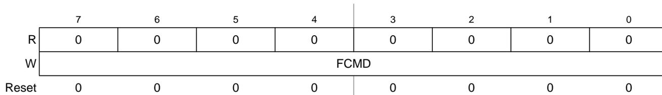
**Figure 4-10. Flash and EEPROM Command Register (FCMD)**
