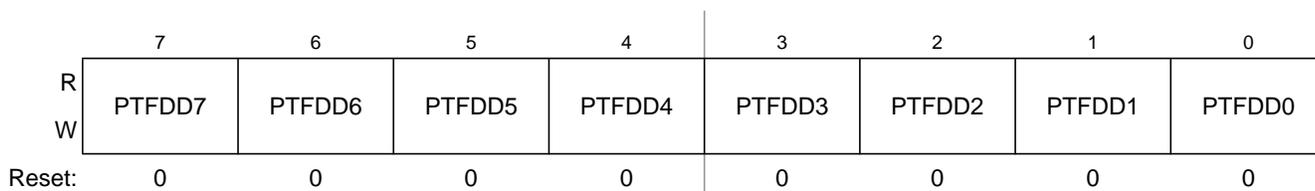
Figure 6-38. Port F Data Direction Register (PTFDD)
