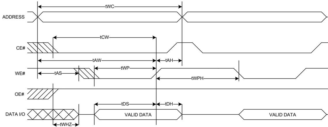
**Write Cycle 2 CE# Controlled, OE# High During Write**
