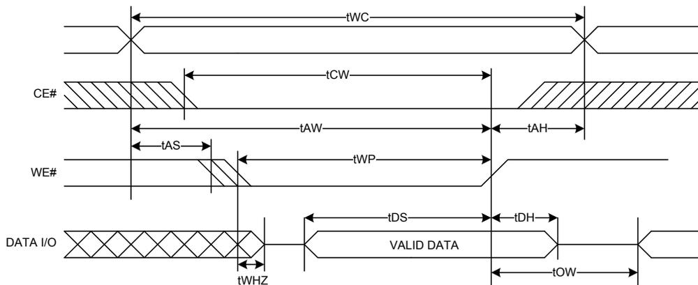
**Note:**  $t_{WP}$  must be adjusted such that  $t_{WP} > t_{WHZ} + t_{DS}$
