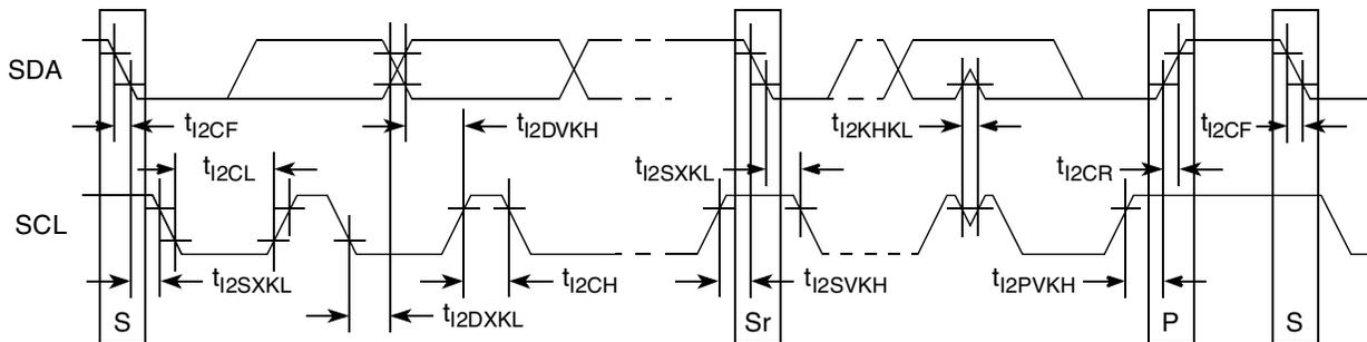
**Figure 38. I<sup>2</sup>C Bus AC Timing Diagram**
