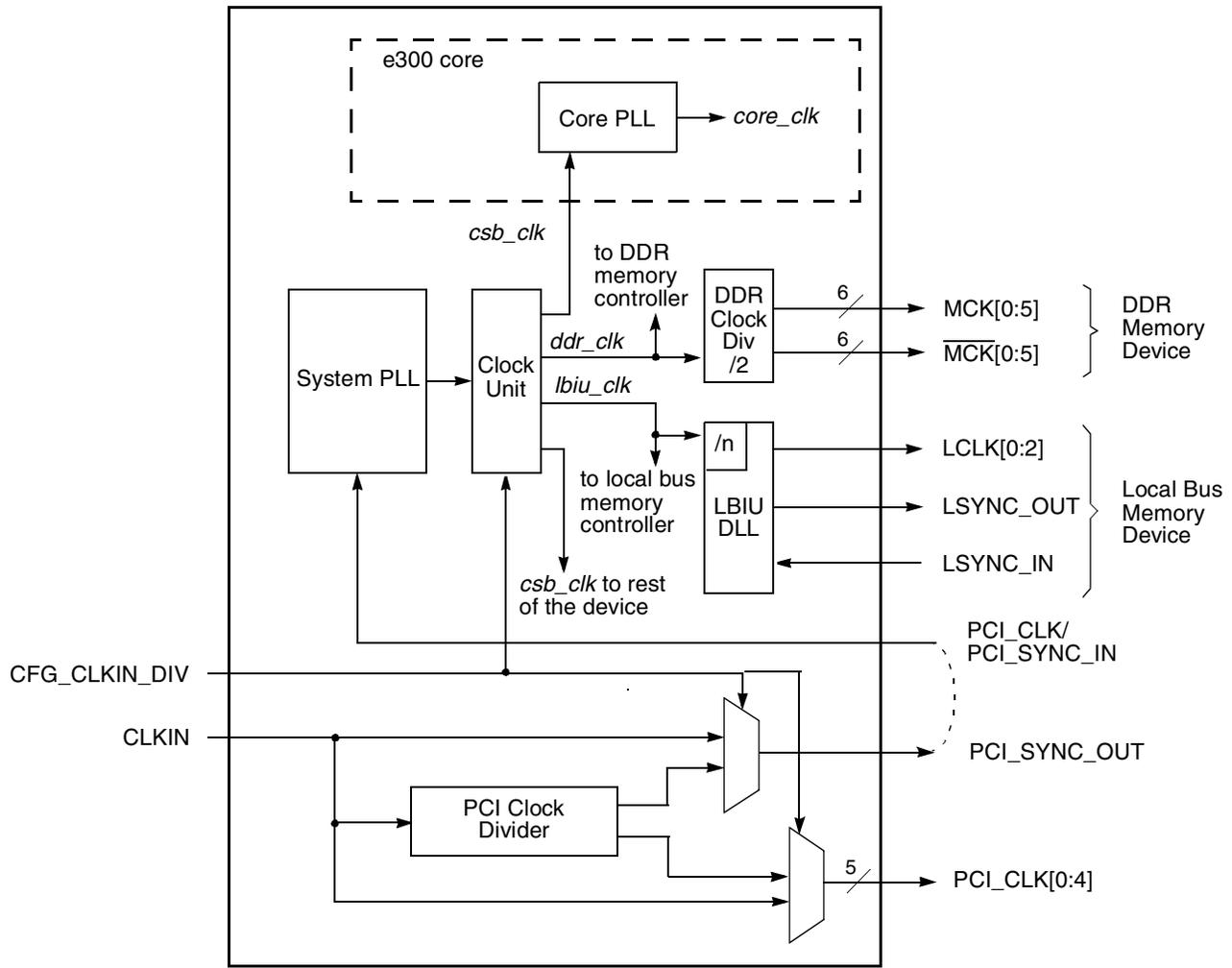
**Figure 64. Clock Subsystem**
