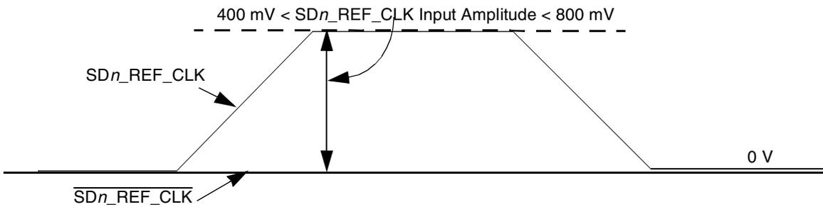
**Figure 55. Single-Ended Reference Clock Input DC Requirements**
