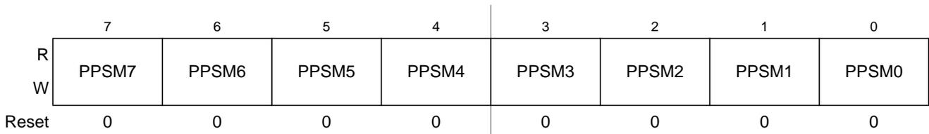
Figure 23-37. Port M Polarity Select Register (PPSM)
