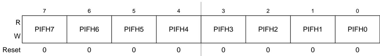
Figure 22-55. Port H Interrupt Flag Register (PIFH)
