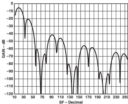
Figure 24. 60 Hz Normal Mode Rejection vs. SF
