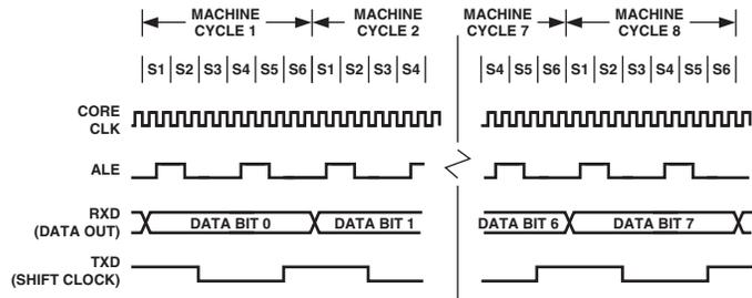
Figure 39. UART Serial Port Transmission, Mode 0
