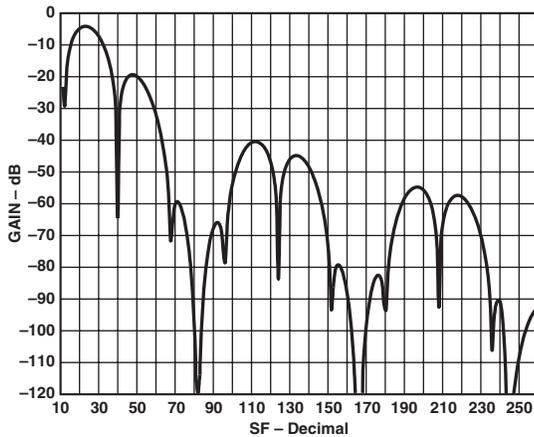
Figure 23. 50 Hz Normal Mode Rejection vs. SF
