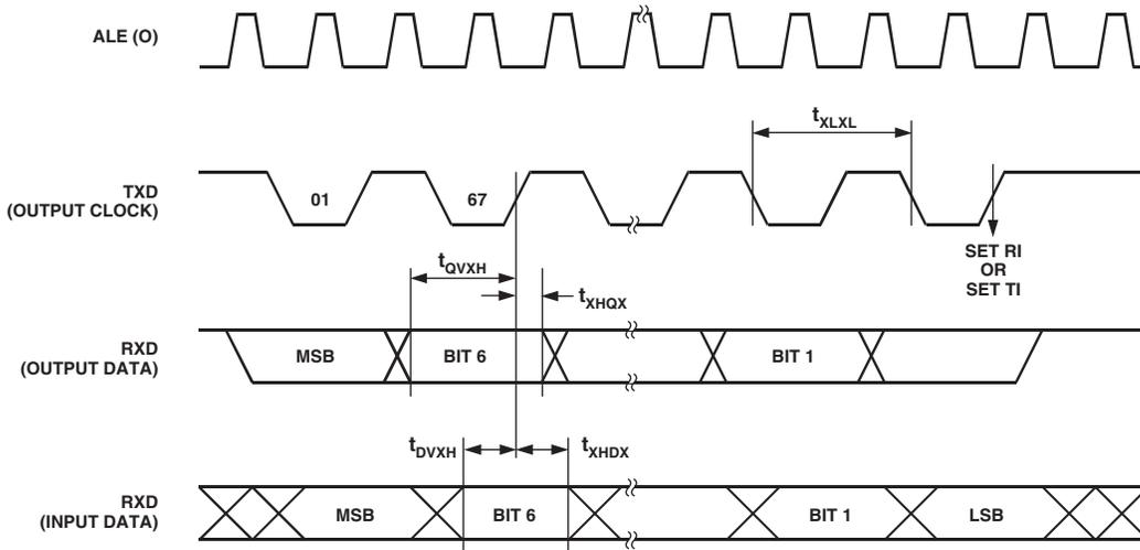
Figure 6. UART Timing in Shift Register Mode
