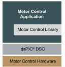
The Motor Control Library contains function blocks that are optimized for the dsPIC33F and dsPIC33E DSC families. All functions in this Motor Control Library have input(s) and output(s), but do not access any of the DSC peripherals. The library functions are designed to be used within an application framework for realizing
