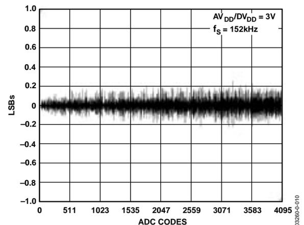
Figure 12. Typical DNL Error,  $V_{DD} = 3V$
