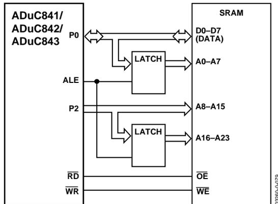
Figure 79. External Data Memory Interface (16 MBytes Address Space)
