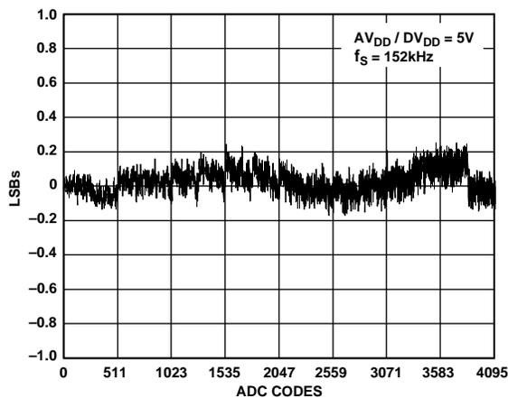
Figure 5. Typical INL Error,  $V_{DD} = 5$  V,  $f_s = 152$  kHz
