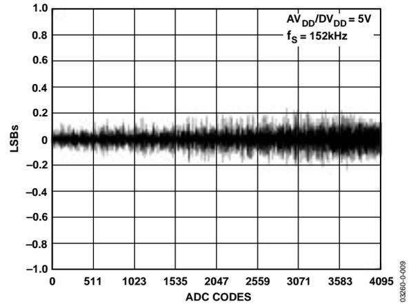
Figure 11. Typical DNL Error,  $V_{DD} = 5V$
