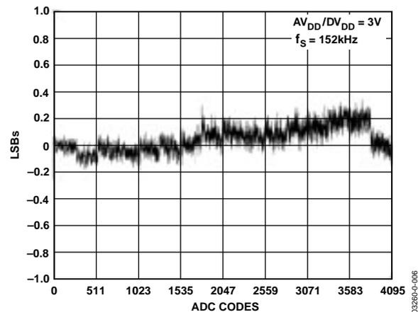
Figure 6. Typical INL Error,  $V_{DD} = 3$  V,  $f_s = 152$  kHz
