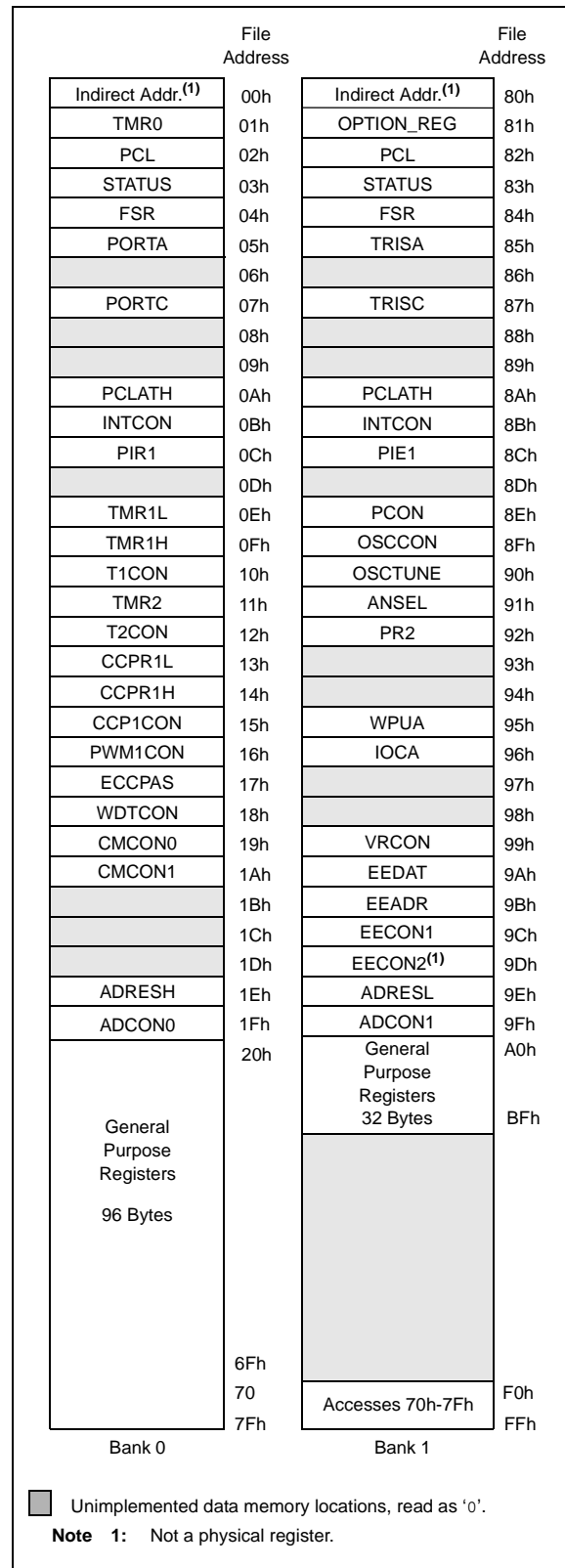
FIGURE 2-2: DATA MEMORY MAP OF THE PIC16F684
