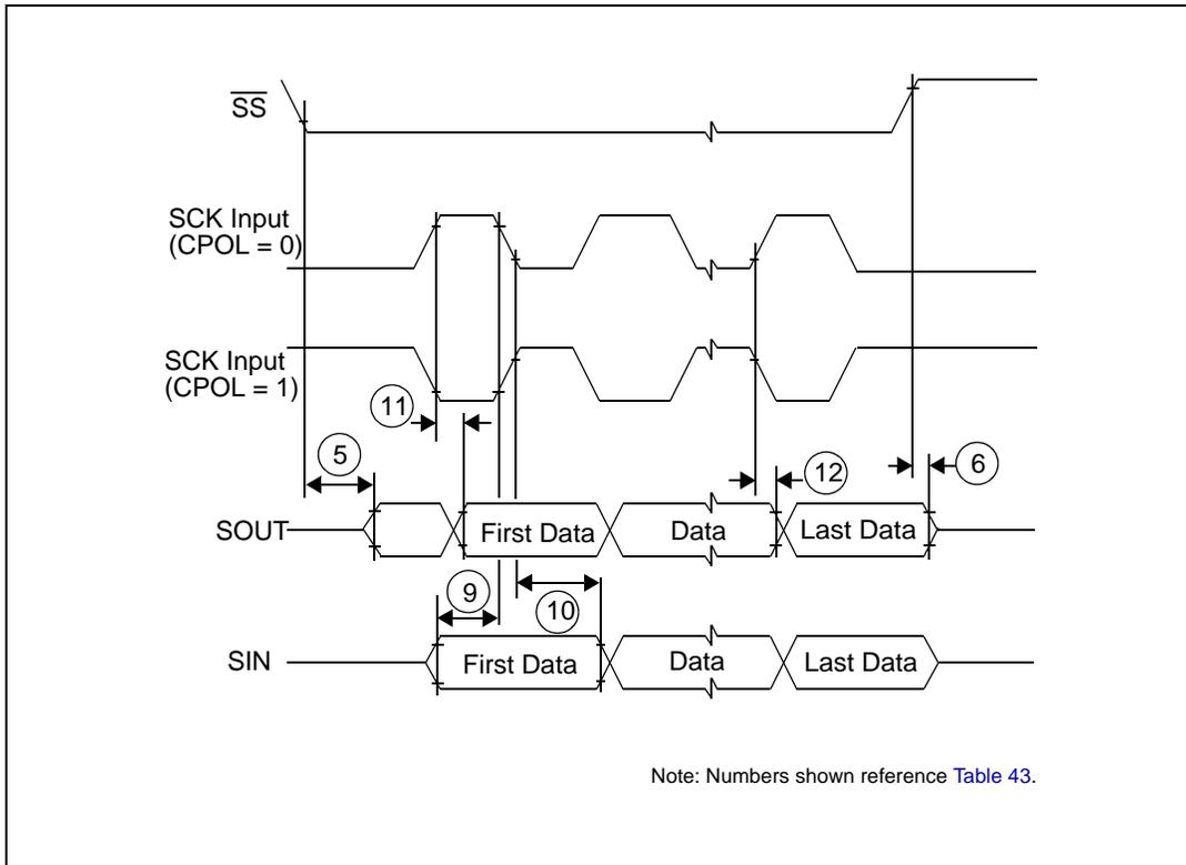
**Figure 19. DSPI classic SPI timing – slave, CPHA = 1**
