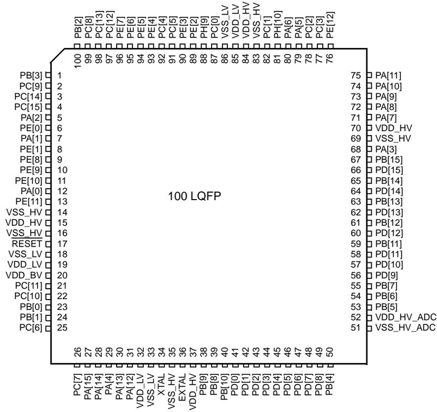
Figure 2. 100 LQFP pin configuration (top view)
