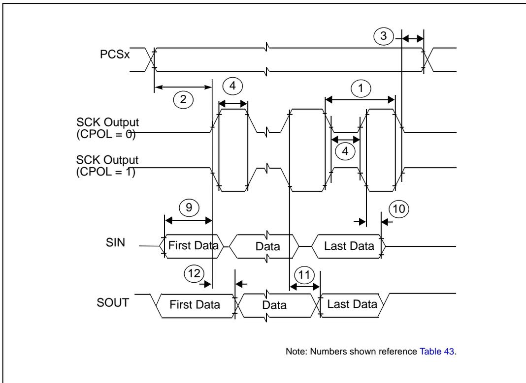
**Figure 20. DSPI modified transfer format timing – master, CPHA = 0**
