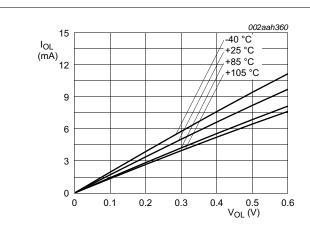
Conditions: V<sub>DD(REG)(3V3)</sub> = V<sub>DD(IO)</sub> = 3.3 V; normal-drive; EHD = 0x0.
