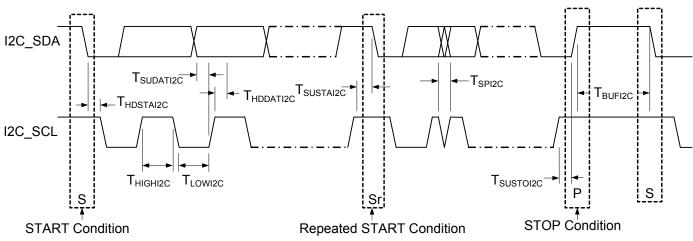
Figure 10. Definition for Timing for Fast or Standard Mode on the I<sup>2</sup>C Bus
