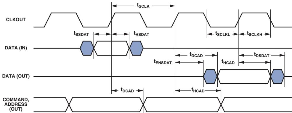
NOTE: COMMAND =  $\overline{SRAS}$ ,  $\overline{SCAS}$ ,  $\overline{SWE}$ ,  $\overline{SDQM}$ ,  $\overline{SMS}$ , SA10, SCKE.
