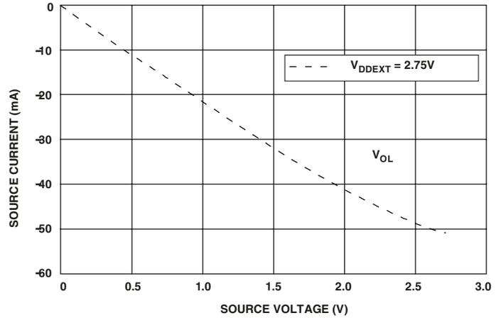
Figure 42. Drive Current E (Low  $V_{DDEXT}$ )
