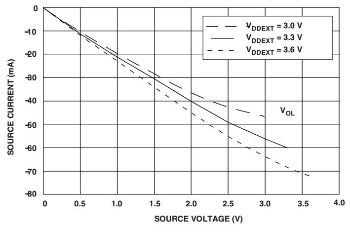
Figure 43. Drive Current E (High  $V_{DDEXT}$ )
