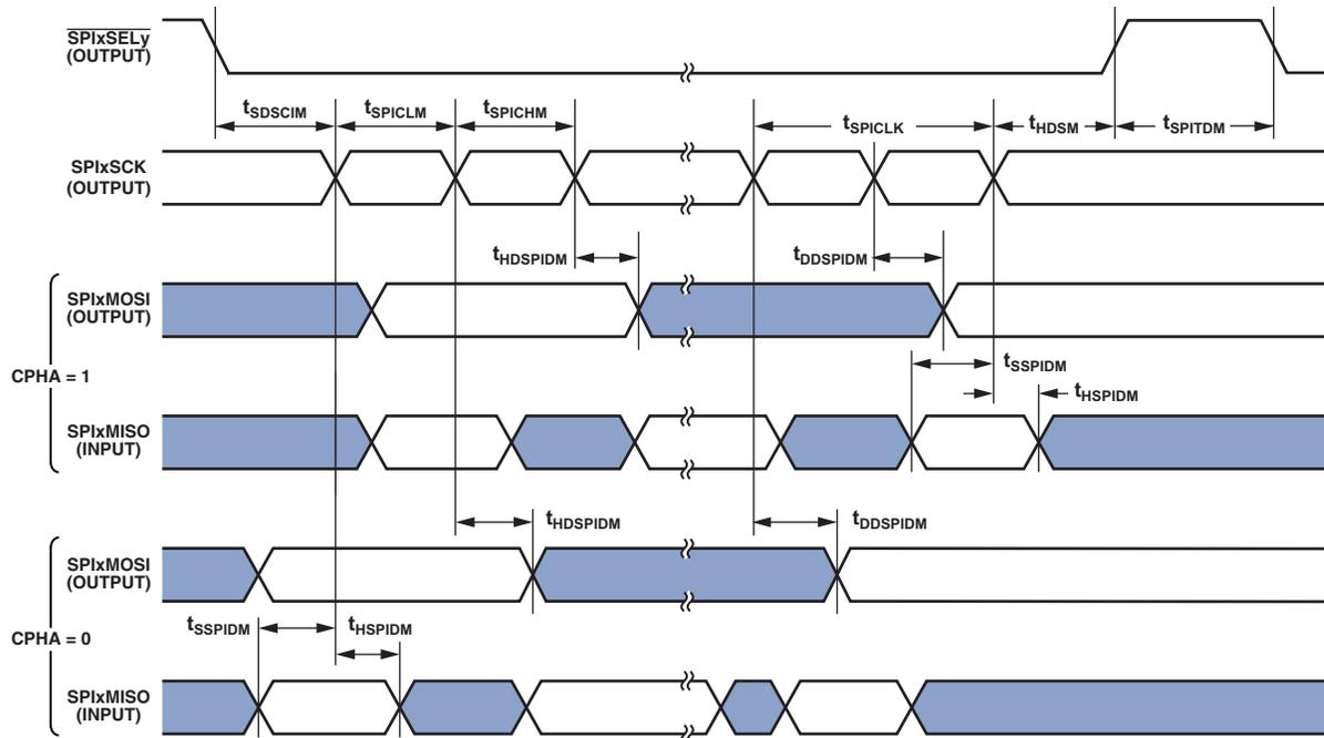
Figure 28. Serial Peripheral Interface (SPI) Ports—Master Timing
