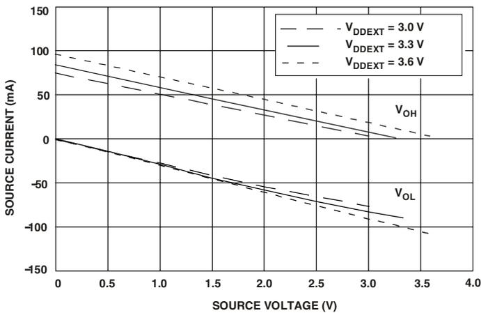
Figure 41. Drive Current D (High  $V_{DDEXT}$ )
