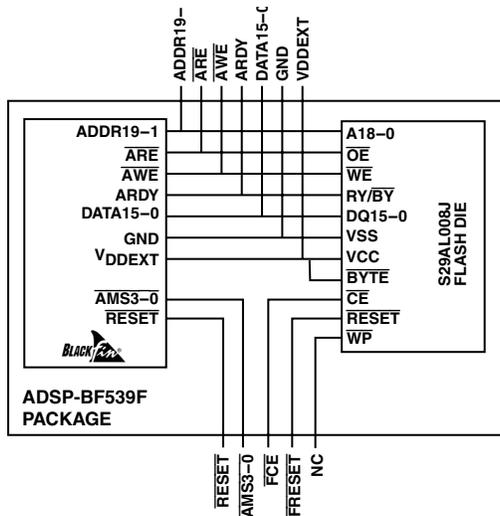
Figure 4. Internal Connection of Flash Memory (ADSP-BF539F8)
