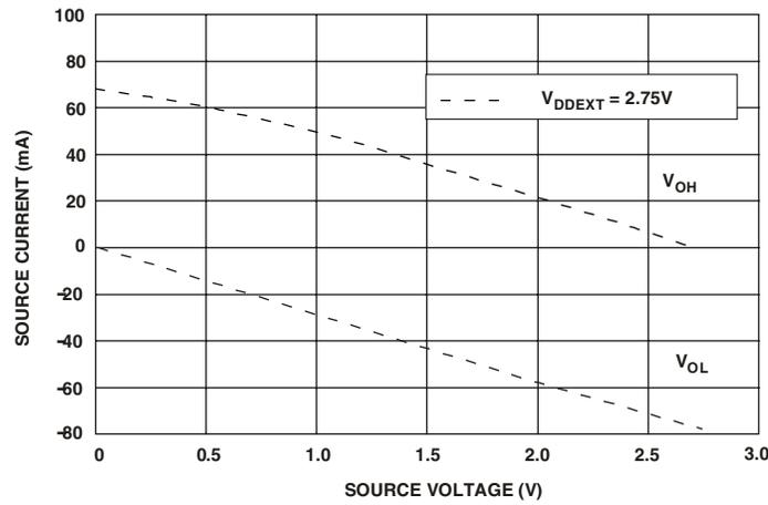
Figure 40. Drive Current D (Low  $V_{DDEXT}$ )
