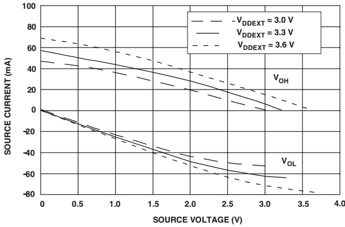
Figure 39. Drive Current C (High  $V_{DDEXT}$ )
