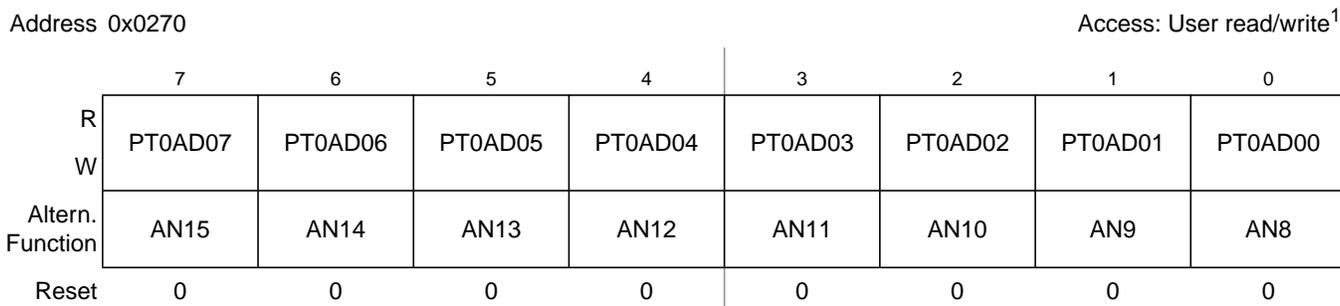
Figure 2-64. Port AD0 Data Register 0 (PT0AD0)
