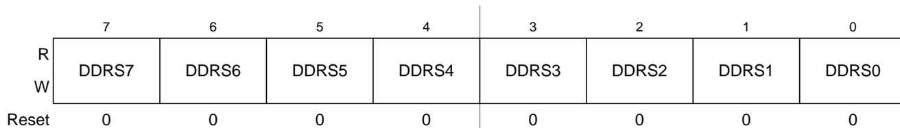
**Figure 2-26. Port S Data Direction Register (DDRS)**
