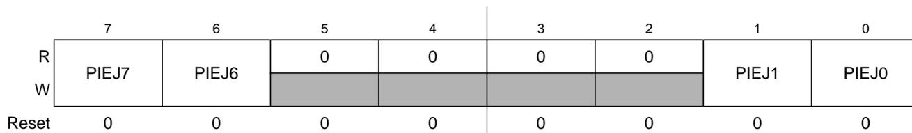
**Figure 2-62. Port J Interrupt Enable Register (PIEJ)**
