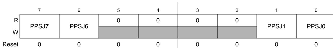
**Figure 2-61. Port J Polarity Select Register (PPSJ)**
