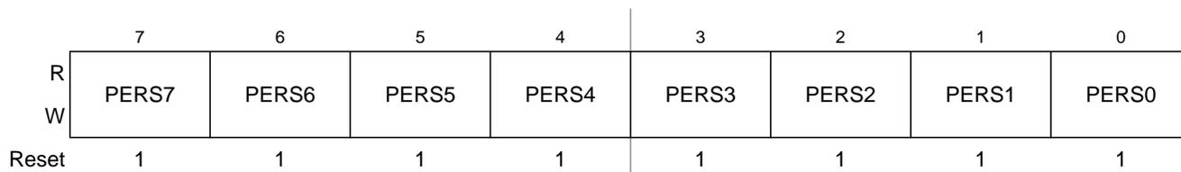
**Figure 2-28. Port S Pull Device Enable Register (PERS)**
