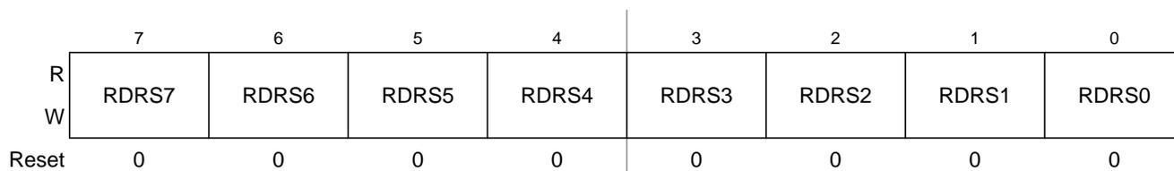
**Figure 2-27. Port S Reduced Drive Register (RDRS)**
