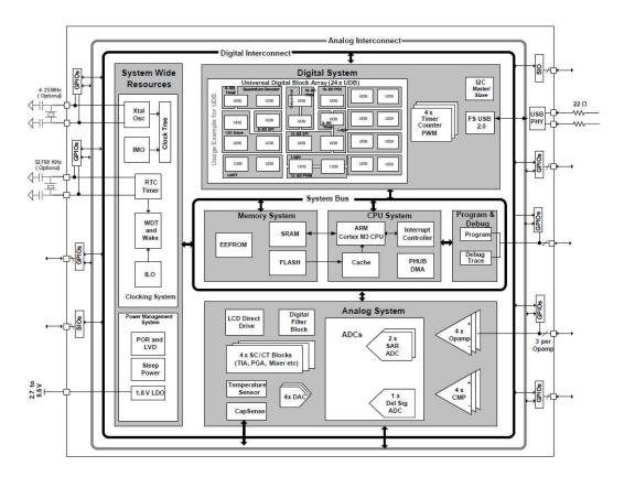
The device used on the DLP-2232H-PSOC5 is the Cypress PSoC® 5 CY8C5588AXI-060. It contains the following:
