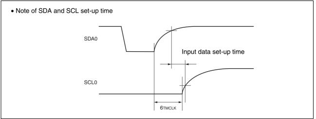
The rating of the input data set-up time in the device connected to the bus cannot be satisfied depending on the load capacitance or pull-up resistor.
