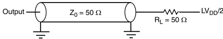
**Figure 13. eTSEC AC Test Load**
