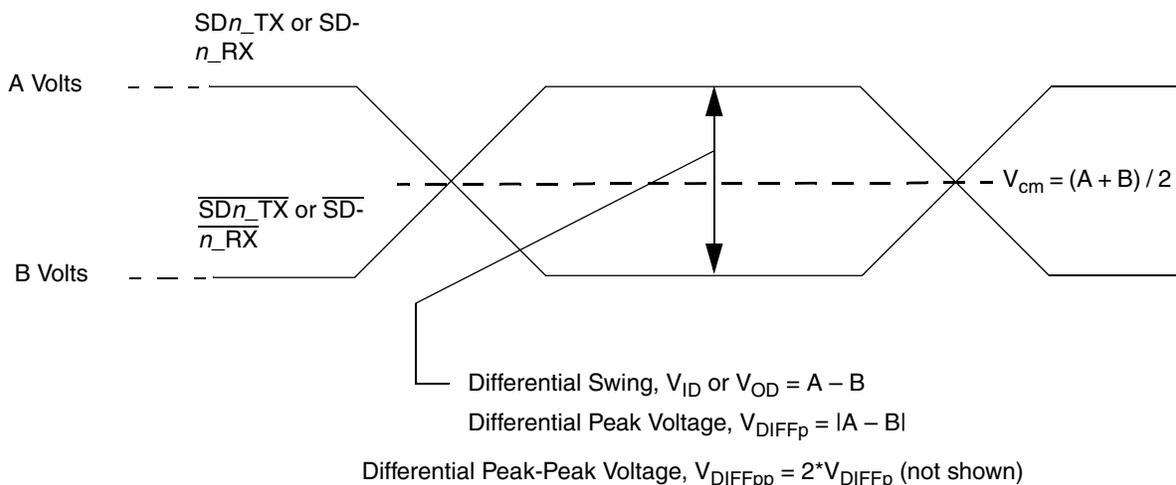
**Figure 40. Differential Voltage Definitions for Transmitter or Receiver**
