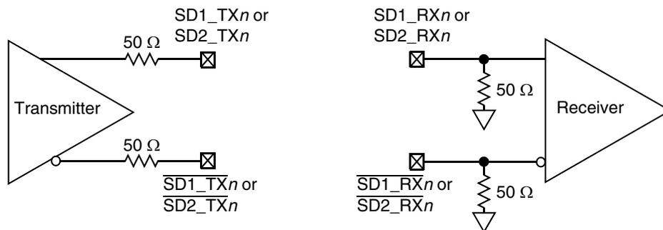
**Figure 51. SerDes Transmitter and Receiver Reference Circuits**
