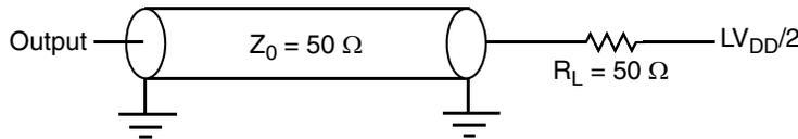
**Figure 20. eTSEC AC Test Load**
