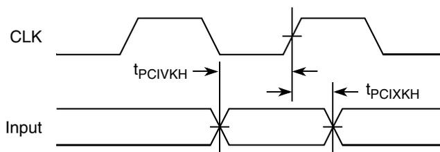
Figure 38. PCI Input AC Timing Measurement Conditions
