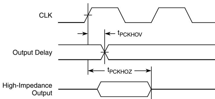
Figure 39. PCI Output AC Timing Measurement Condition
