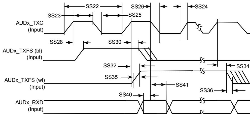
Figure 43. SSI Receiver External Clock Timing Diagram
