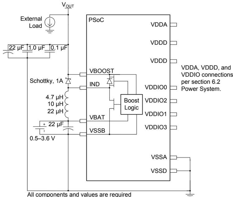
The switching frequency is set to 400 kHz using an oscillator integrated into the boost converter. The boost converter can be operated in two different modes: active and standby. Active mode is the normal mode of operation where the boost regulator
