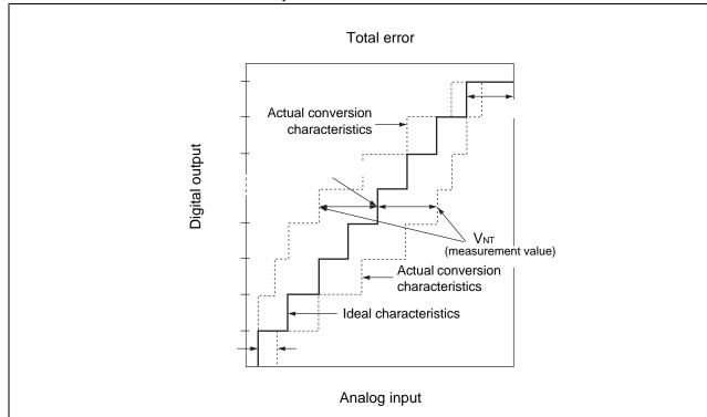
$$\frac{\text{1LSB'}}{\text{(Ideal value)}} = \frac{\text{AVRH} - \text{AVss}}{1024} \text{ [V]} \quad \text{Total error of digital output N} = \frac{\text{V}_{\text{NT}} - \{1 \text{ LSB'} \times (N-1) + 0.5 \text{ LSB'}\}}{1 \text{ LSB'}}$$
