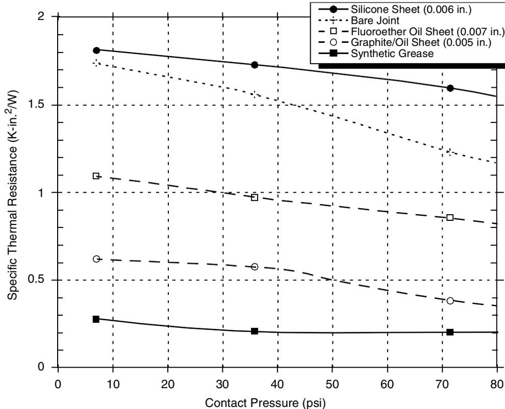
**Figure 25. Thermal Performance of Select Thermal Interface Material**
