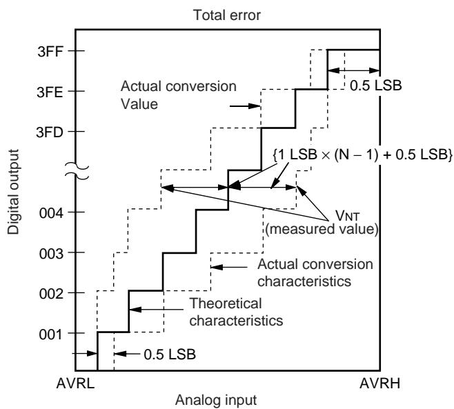
$$1 \text{ LSB} = (\text{Theoretical value}) \frac{\text{AVRH} - \text{AVRL}}{1024} [\text{V}]$$
