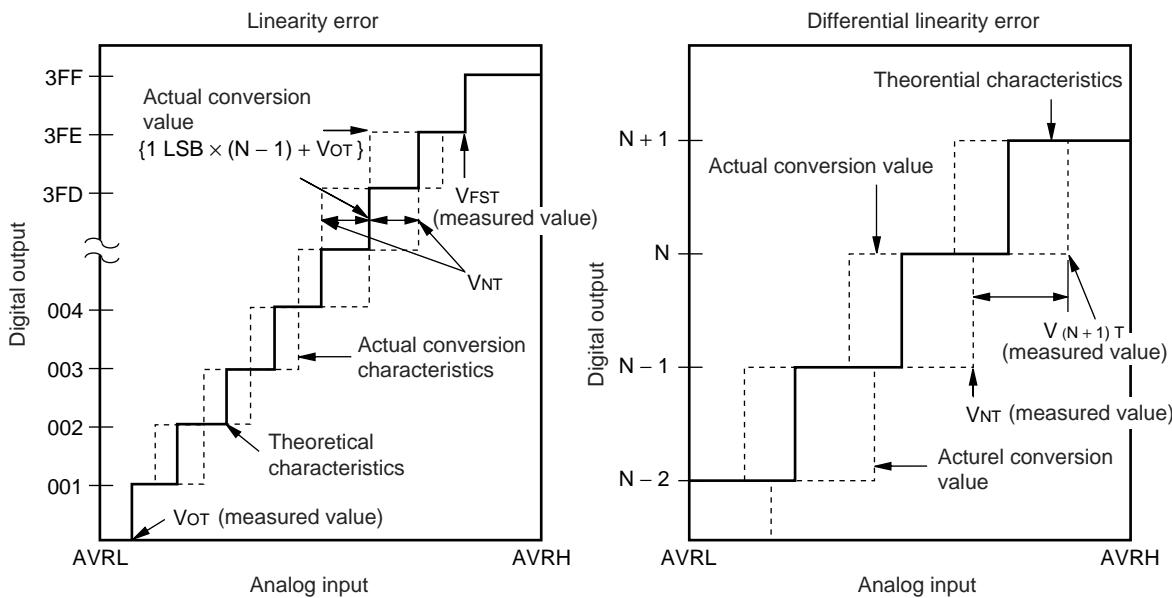
$$\text{Linearity error of digital output } N = \frac{V_{NT} - \{1 \text{ LSB} \times (N - 1) + V_{OT}\}}{1 \text{ LSB}} \text{ [LSB]}$$
