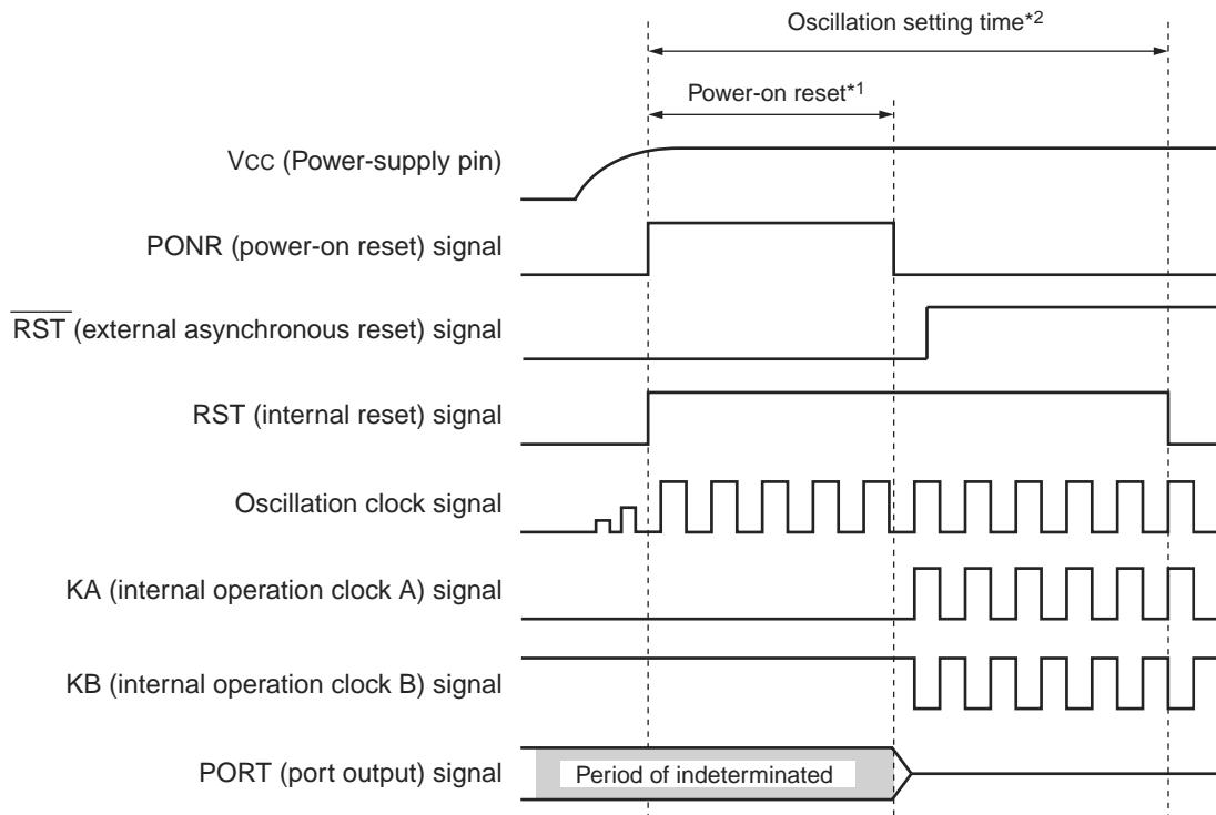
\*1 : Power-on reset time : "Period of clock frequency" × 2<sup>17</sup> (Clock frequency of 16 MHz : 8.19 ms)
