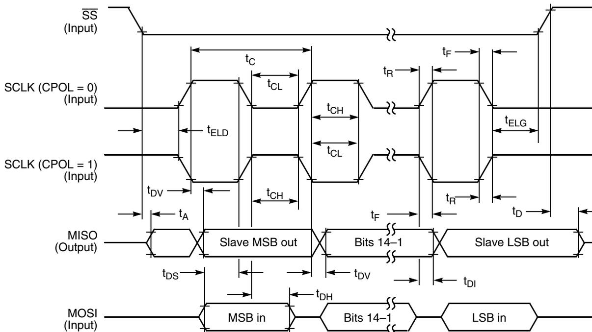
Figure 23. SPI Slave Timing (CPHA = 1)
