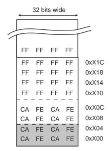
Step 3: Flash array after programming a second 64-bit data at address 0xX00 (write latch buffer + WP)
