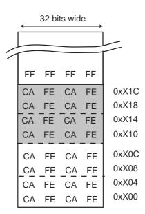
Step 4: Flash array after programming a 128-bit data word at address 0xX10 (write latch buffer + WP)
