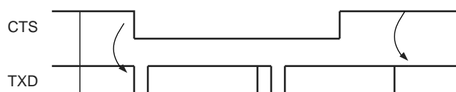
Figure 36-28. Transmitter Behavior when Operating with Hardware Handshaking
