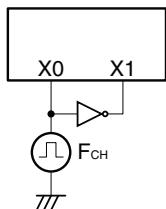
■ Input waveform generated when an external clock (subclock) is used
