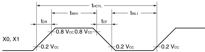
■ Figure of main clock input port external connection
