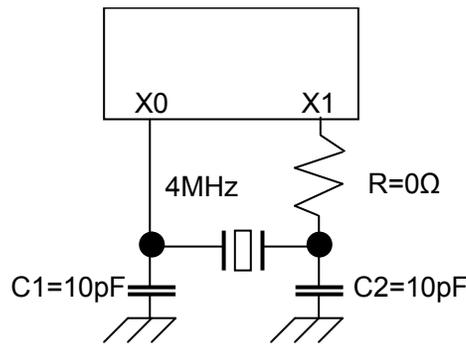
**Note:** As to the product with its clock supervisor's initial value is "ON", when the oscillator is unable to start within 20ms from the stop state the clock supervisor will detect the oscillation stop. As a result, the CPU moves to the fail safe operation.
