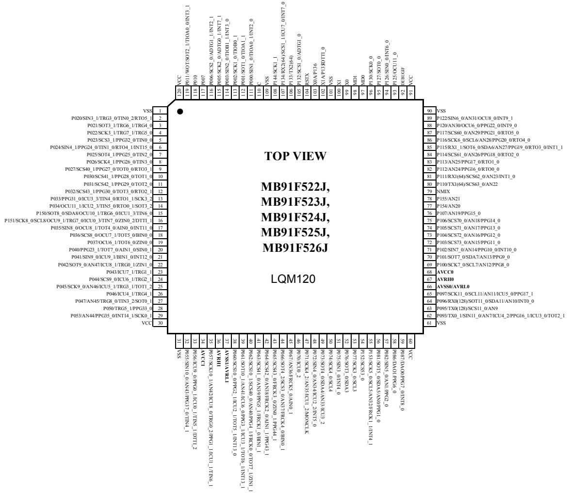
\* In a single clock product, pin 102 and pin 103 are the general-purpose ports.
