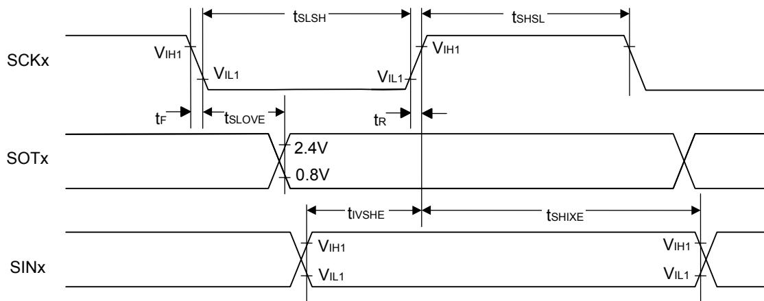
**(4-2) UART (Asynchronous serial interface) timing**
