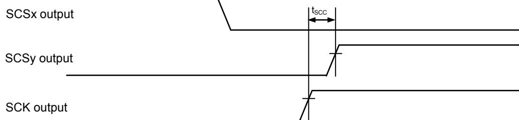
When Serial chip select is used , Serial clock output mark level "L",
