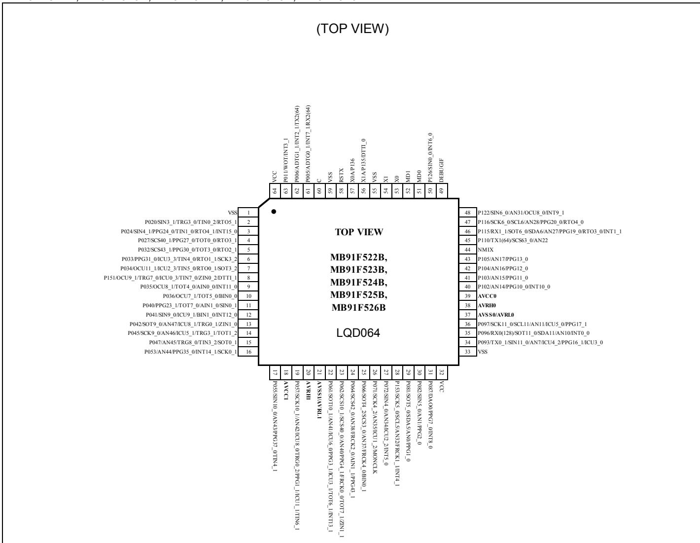
\* In a single clock product, pin 56 and pin 57 are the general-purpose ports.
