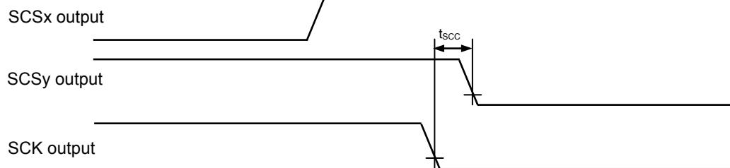
When Serial chip select is used , Serial clock output mark level "H"
